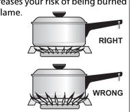
**For most cooking**, start on the highest control setting and then turn to a lower one to complete the process. Use the chart below as a guide for determining proper flame size for various types of cooking. The size and type of utensil used and the amount of food being cooked will influence the setting needed for cooking.
